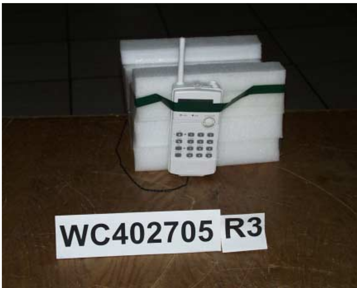
Figure 1: Picture of DUT on test table, showing class 2 transformer connected.
