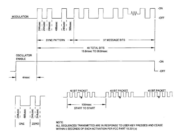
TRANSMITTER MODULATION & TIMING
