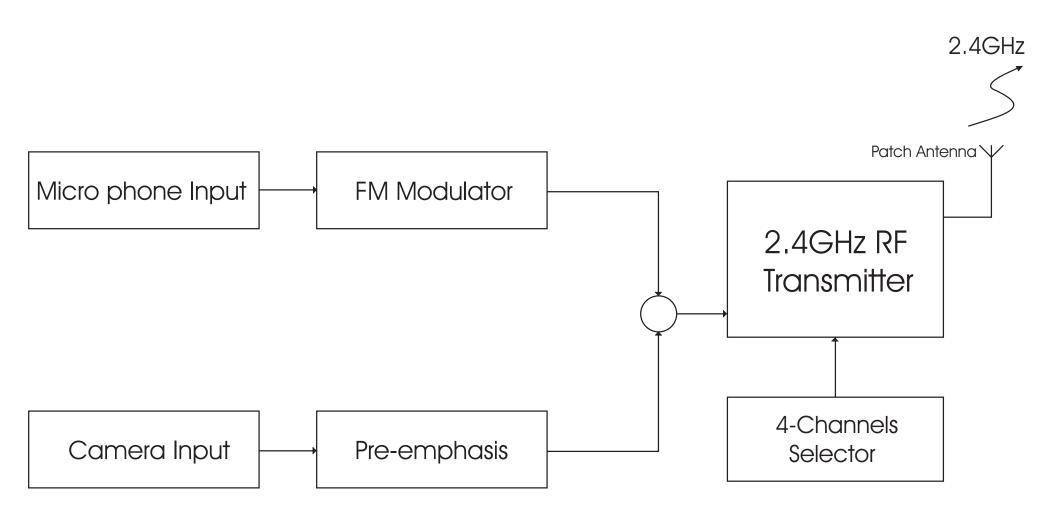
Block Diagram for Indoor/Outdoor Color Video Camera With Built-in 2.4 GHz Transmitter (XC18A)
