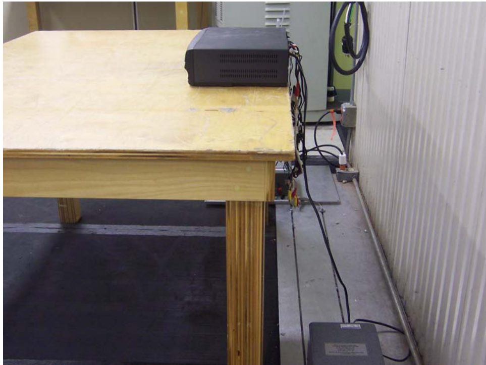
Transmitter, Conducted Emissions, Left Side Setup View
