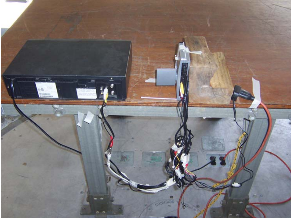
Transmitter, Radiated Emissions, Fundamental and Harmonics, Y-Axis Setup
