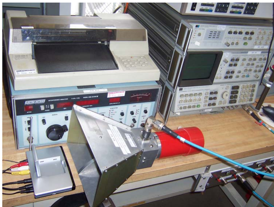
Transmitter, Occupied Bandwidth, Test Setup
