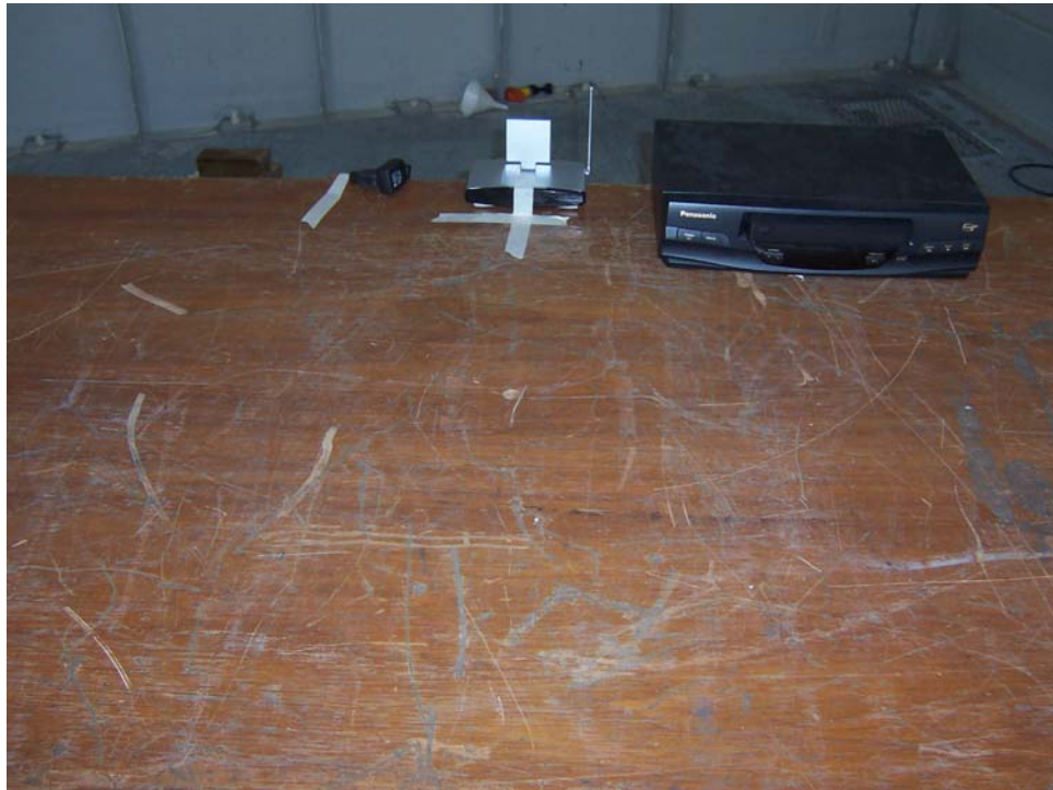
Transmitter, Radiated Emissions, Spurious Case, Front View Setup
