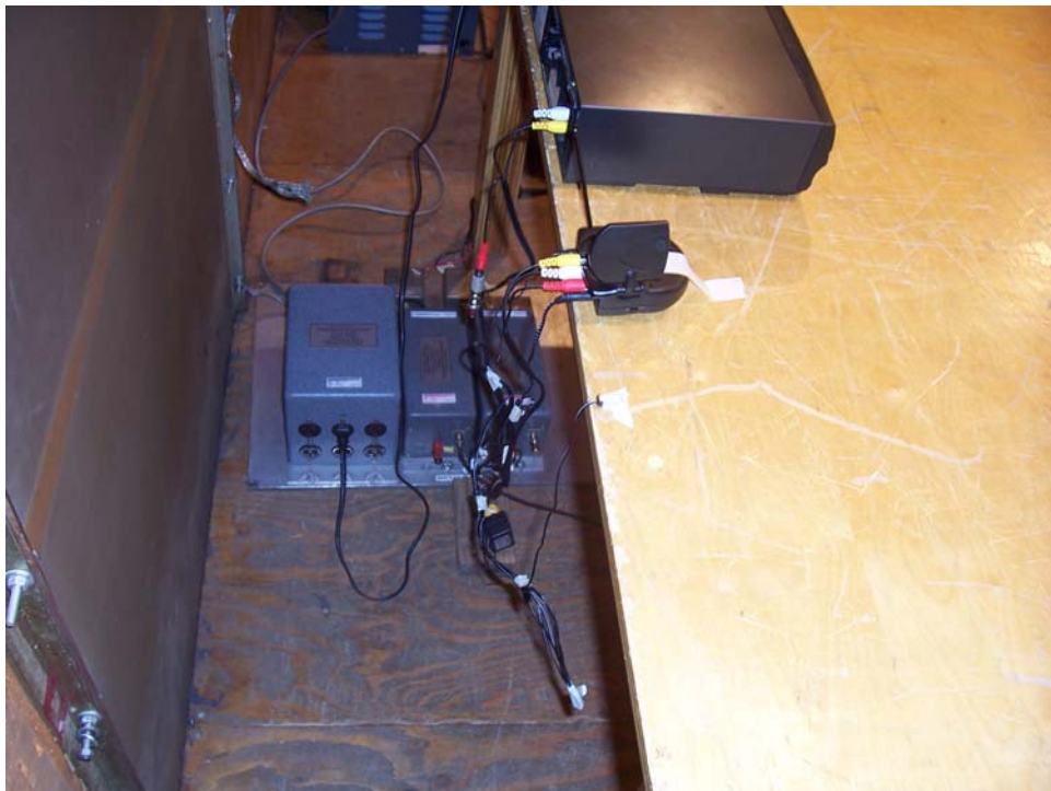
Conducted Emissions, Rear Test Setup
