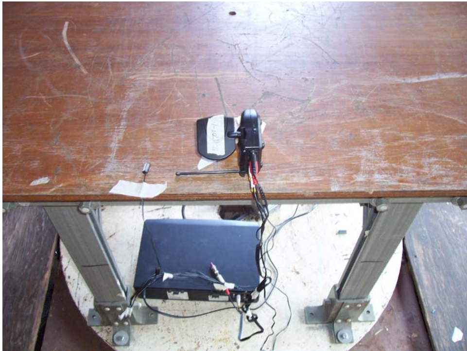
Radiated Emissions, Y-Axis, Transmitter Test Setup
