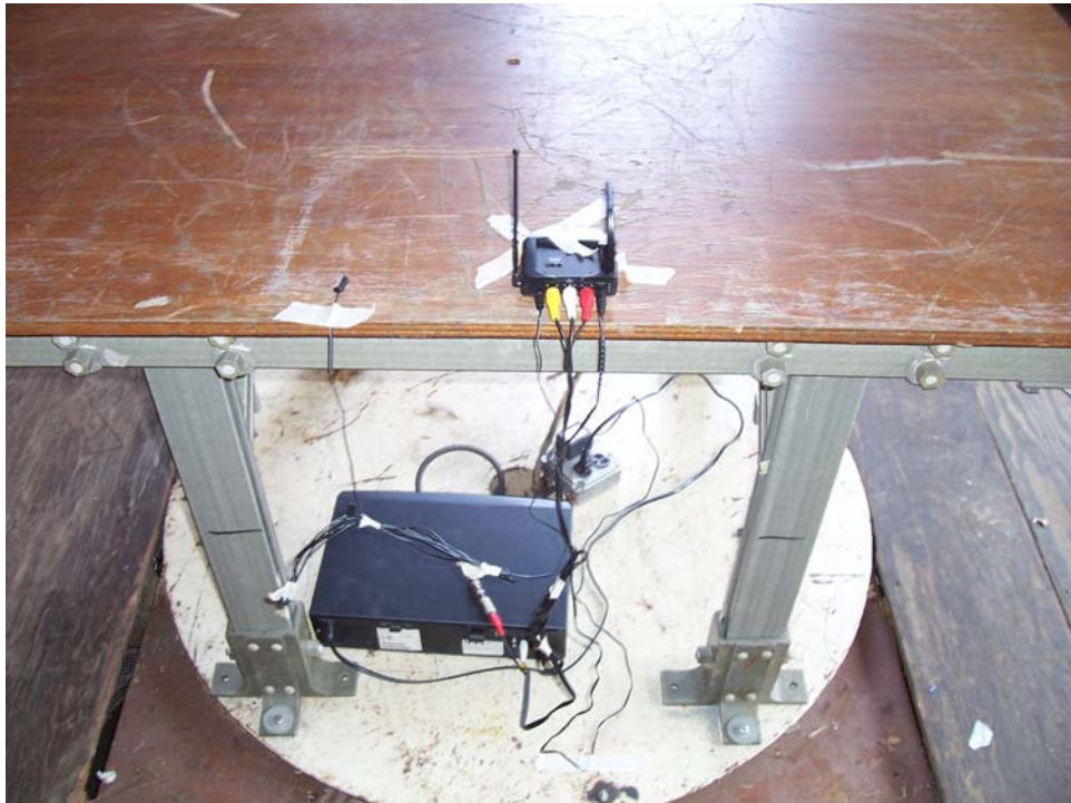
Radiated Emissions, X-Axis, Transmitter Test Setup
