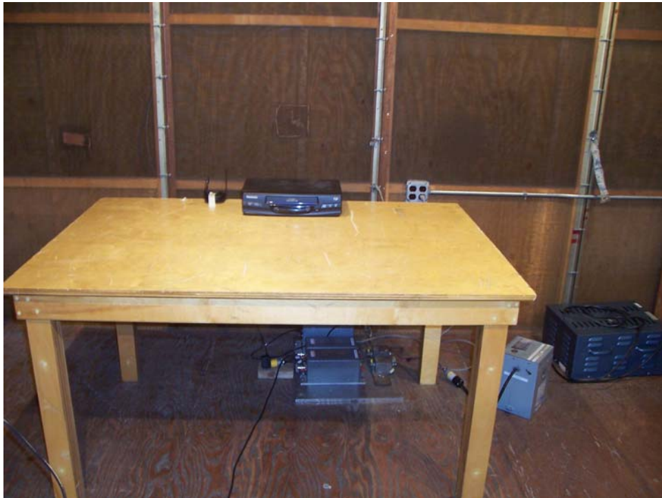
Conducted Emissions, Test Setup
