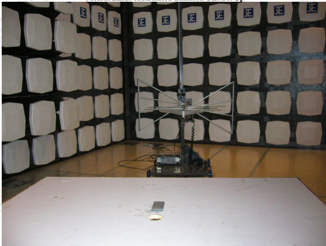
Measurement of Radiated Emission Test Set Up
