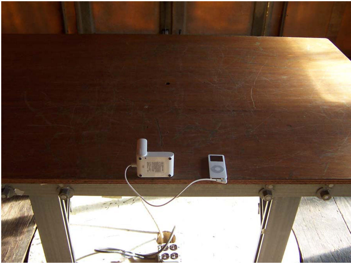
Radiated Emissions Test Setup (Y-axis)
