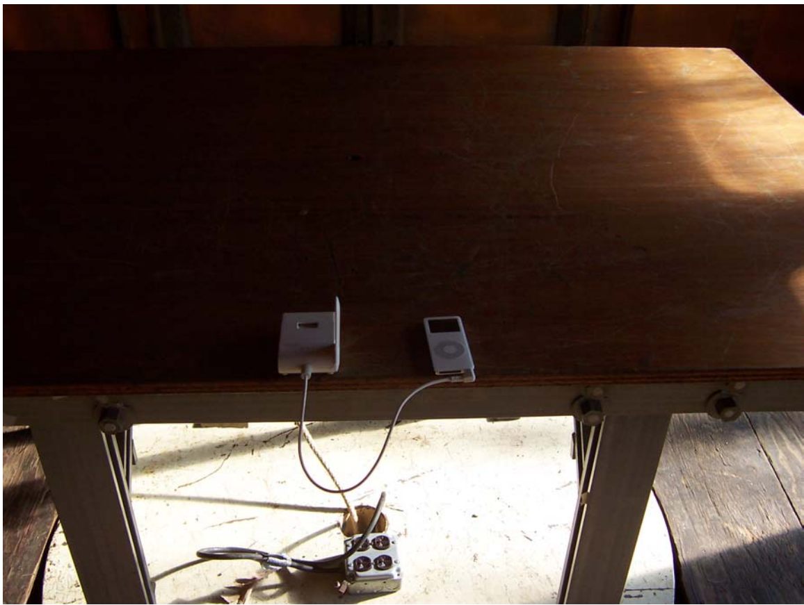
Radiated Emissions Test Setup (X-axis)
