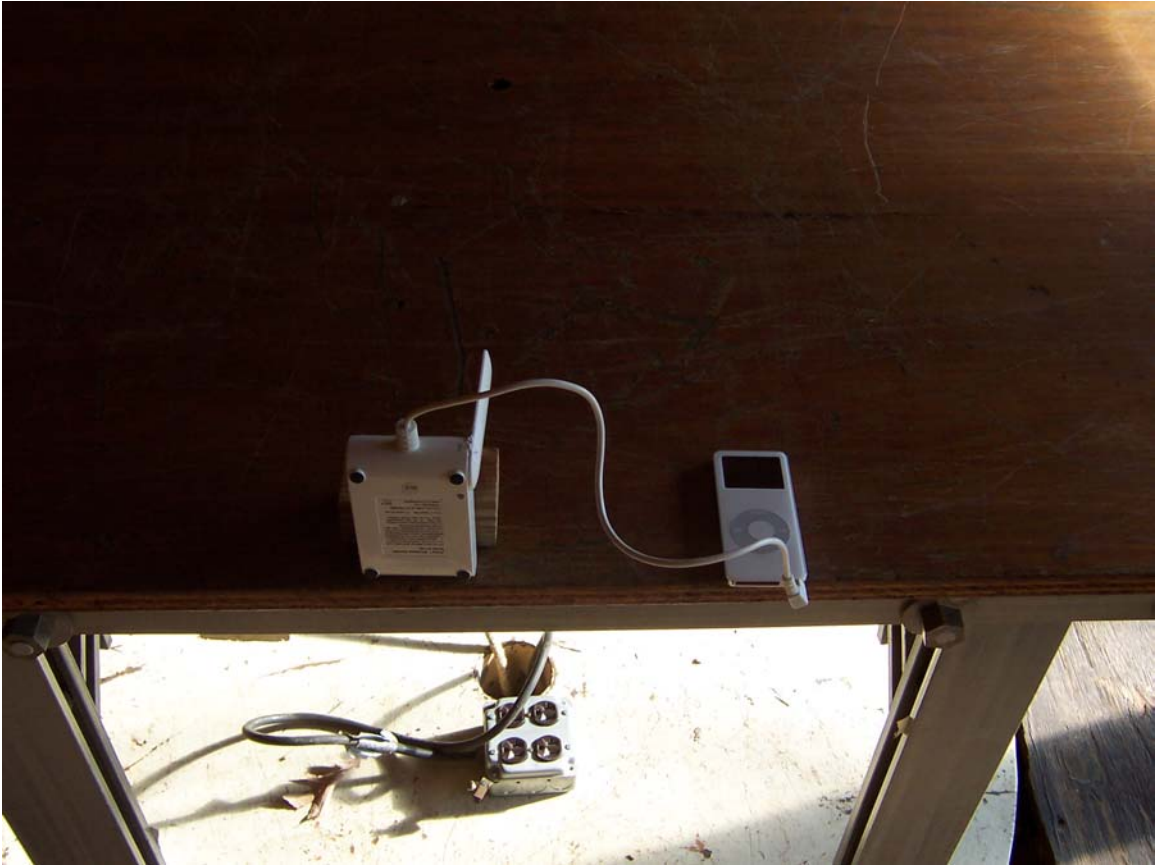
Radiated Emissions Test Setup (Z-axis)
