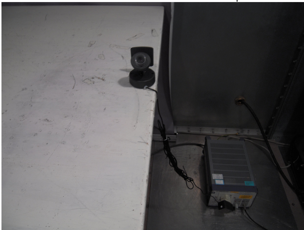
Measurement of Conducted Emission Test Set Up
