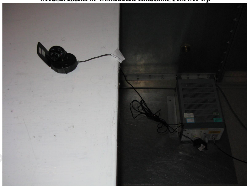
Measurement of Conducted Emission Test Set Up
