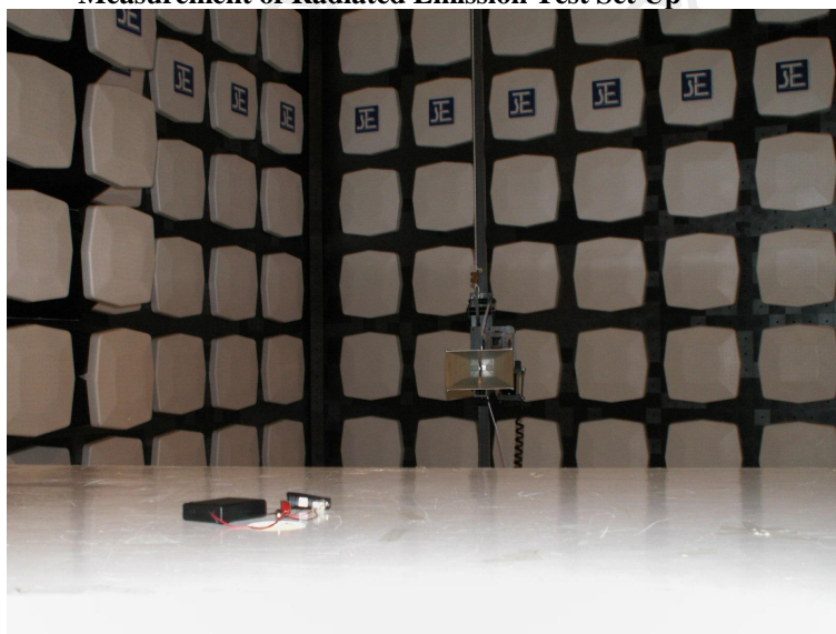
Measurement of Radiated Emission Test Set Up
