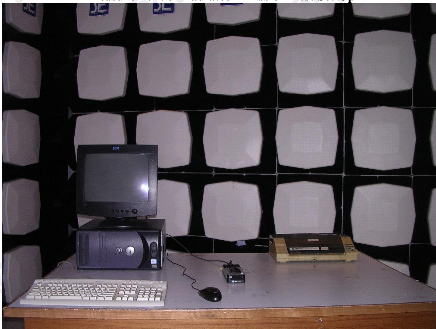
Measurement of Radiated Emission Test Set Up
