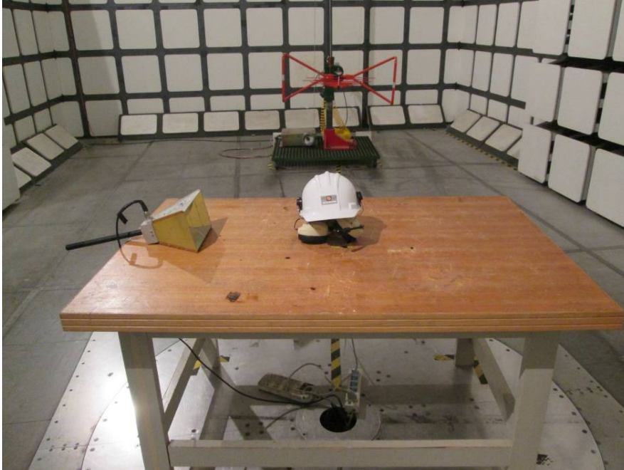
Radiated Emissions – (Below 1 GHz)
