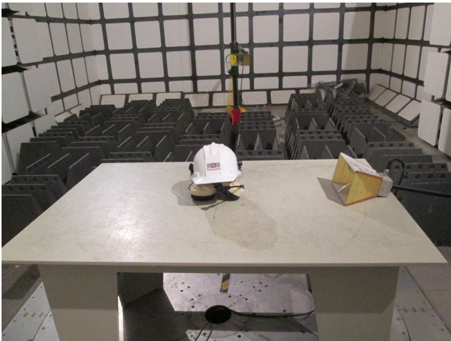
Radiated Emissions – (Above 1 GHz)
