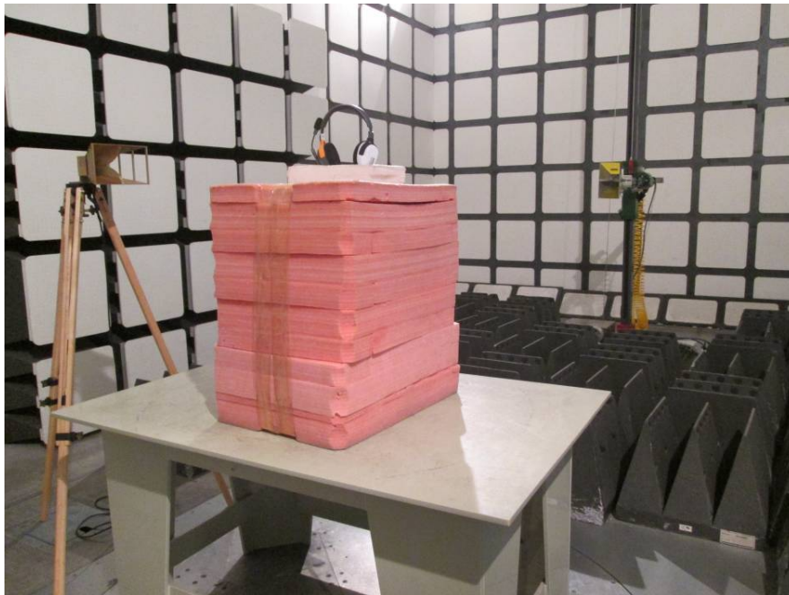
Radiated Emissions View (Above 1 GHz, Model: ComStar Ultralite-RD(ULRD2015))
