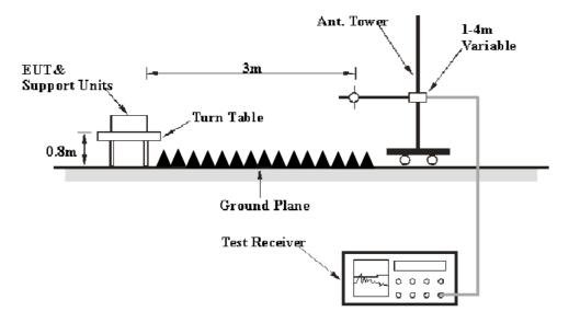
The radiated emission tests were performed in the 3 meters test site, using the setup accordance with the ANSI C63.4 - 2014. The specification used was the FCC  $15\S 15.319(g)$ .
