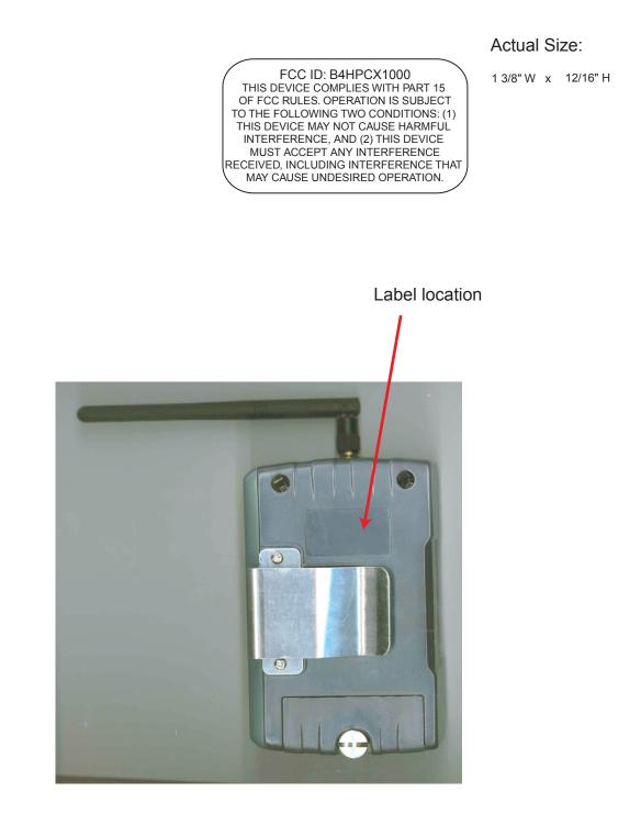
Note:This label will be made from lexan polycarbonate material and will be affixed to the back of the radio chassis, using an aggressive permanent adhesive.
