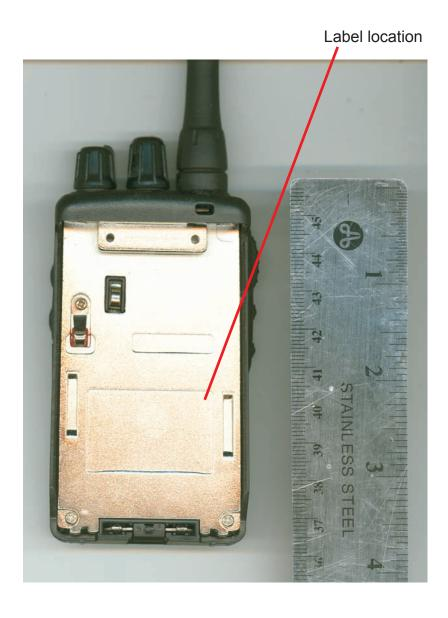
Note: The dimensions of the radio are such that there is limited space to affix FCC label to the exterior. The transceiver length is only 3.5". We will affix label to inside chassis as indicated.
