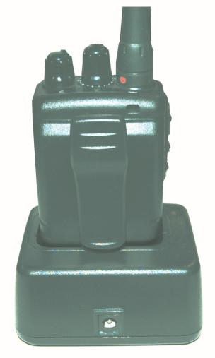
During Battery charging procedure, back of radio below the belt clip area is flush against charger. The FCC label will become damaged or lost if affixed here.
