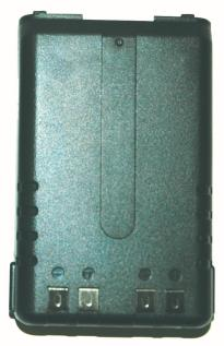
Radio back chassis encapsulates rechargable battery. This assembly is removable. If FCC label is placed here, it could become separated from actual radio and lost.
