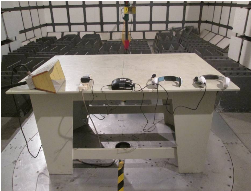
Radiated Emissions – Rear View (Above 1 GHz)
