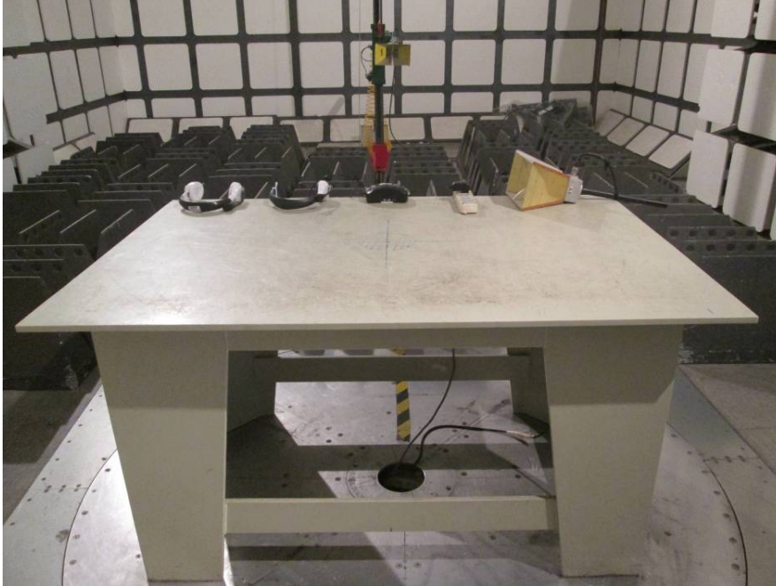
Radiated Emissions – Front View (Above 1 GHz)
