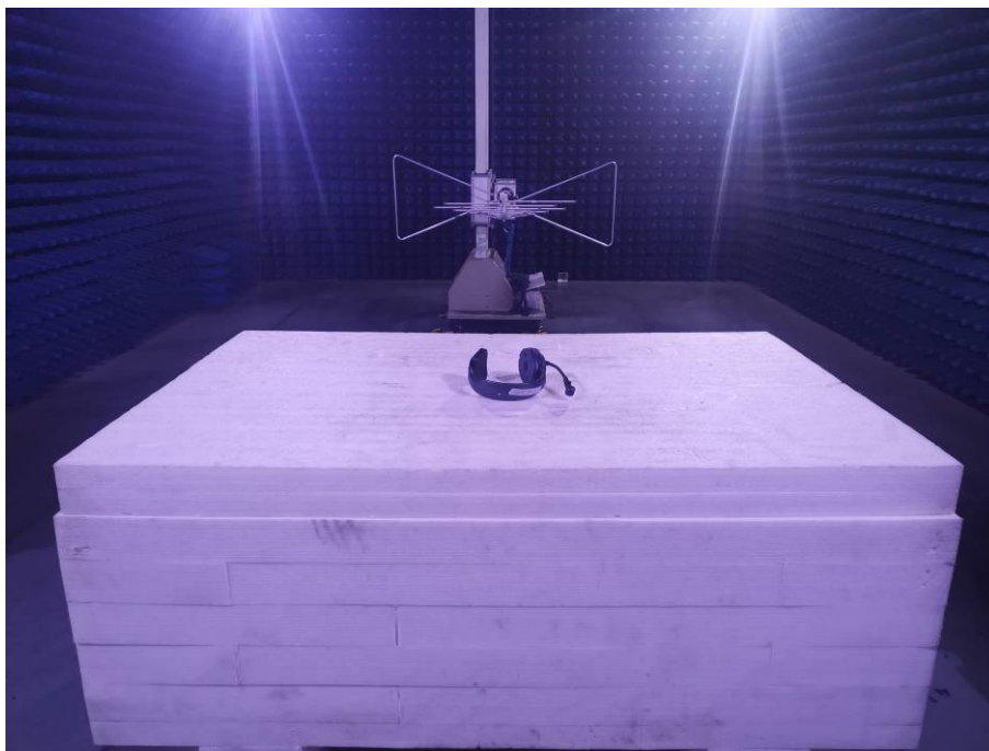
Photo of Radiated Emission Measurement (Above 1G)
