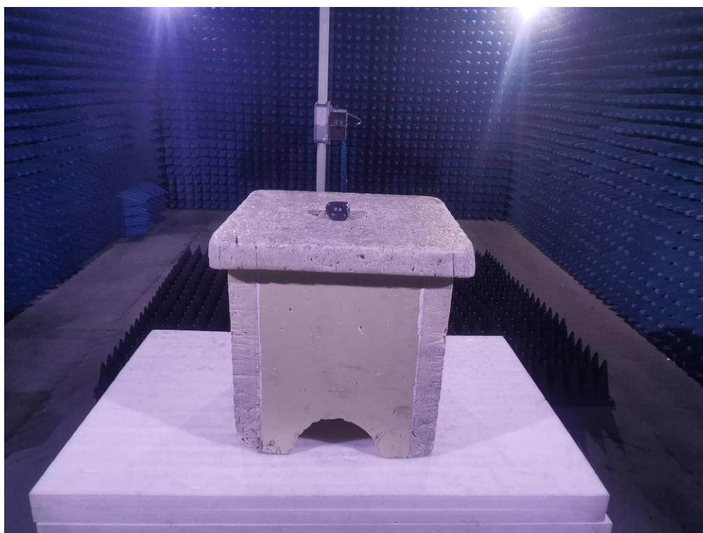
Photo of Radiated Emission Measurement (Above 1G)
