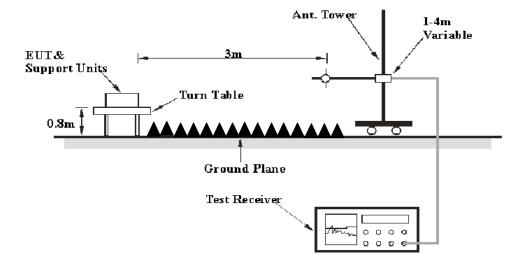
The radiated emission tests were performed in the 3 meters chamber B test site, using the setup accordance with the ANSI C63.17 - 2006. The specification used was the FCC 15.209 and FCC 15.319(g) limits.
