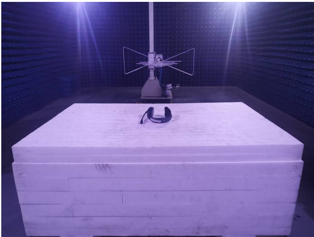
Photo of Radiated Emission Measurement (Above 1G)
