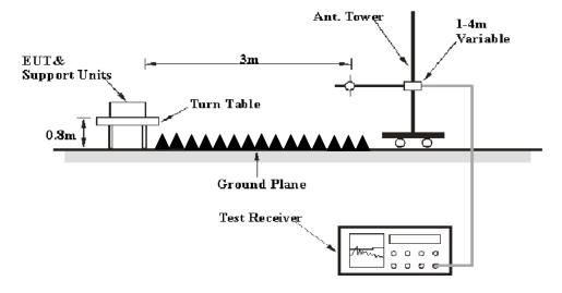
The radiated emission tests were performed in the 3 meters chamber B test site, using the setup accordance with the ANSI C63.17-2006. The specification used was the FCC 15§ 15.319(g).
