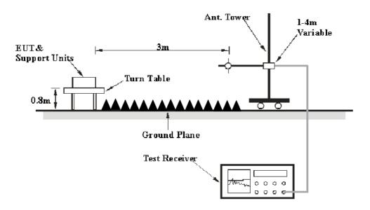
The radiated emission tests were performed in the 3 meters test site, using the setup accordance with the ANSI C63.4 - 2014. The specification used was the FCC 15 15.319(g).
