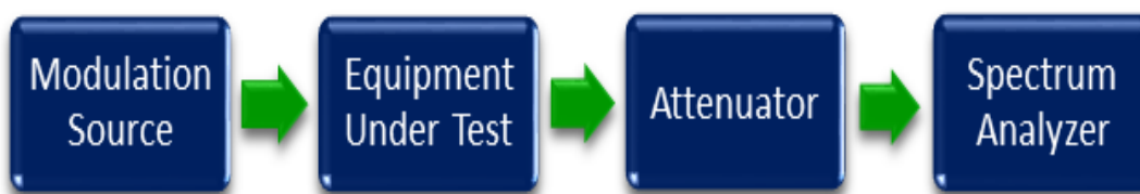
Figure 2: Modulation Characteristics Bandwidth Test Setup
