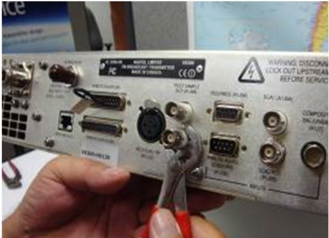
Figure 4-2: Loosening the BNC connector's locking ring
