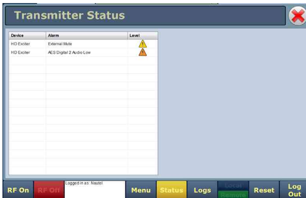
Figure 2.81: Transmitter Status page
