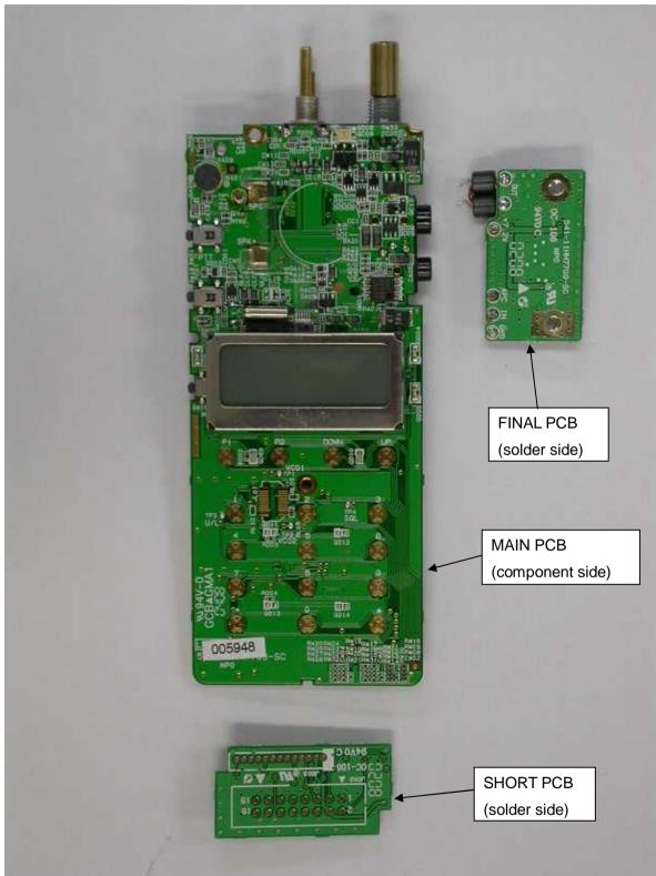
9) MAIN PCB of HH7700 (Component Side View)
