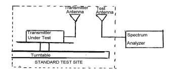
b) Raise and lower the test antenna from 1m to 6 m with the transmitter facing the antenna and record the highest received signal in dB as LVL.
