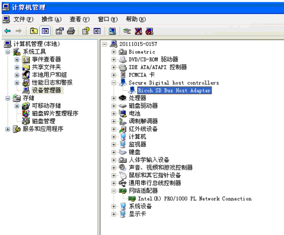
3, Insert DUT into SDIO slot of notebook,then Install driver based on **Ricoh SD Bus Host Adapter** directly.
