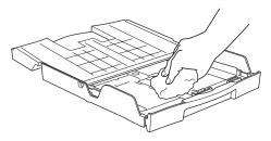
5 Close the output paper tray cover and put the paper tray firmly back in the machine.
