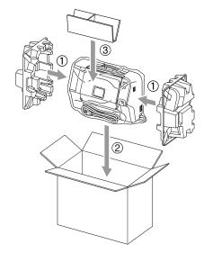
9 Pack the printed materials in the original carton as shown below. Do NOT pack the used ink cartridges in the carton.
