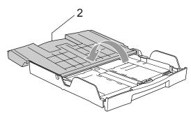
2 If you are using Letter, A4 or Legal size paper, press and hold the universal guide release button (1) as you slide out the front of the paper tray to match the paper size you are using.
