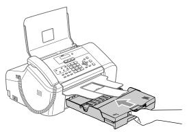
While holding the paper tray in place, pull out the paper support (1) until it clicks and unfold the paper support flap (2).
