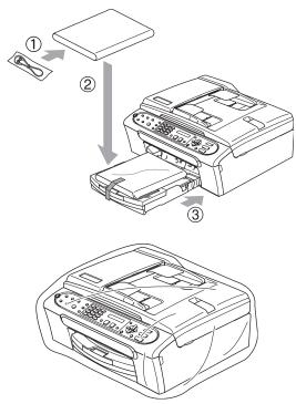
10 Pack the printed materials and additional parts (handset and cords) in the original carton as shown below. Do not pack the used ink cartridges in the carton.
