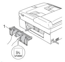
Clean the Paper Pick-up Roller (1) with isopropyl alcohol on a cotton swab.
