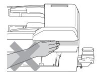
When moving the machine you must lift it from the base, by placing a hand at each side of the unit as shown in the illustration. Do not carry the machine by holding the scanner cover.
