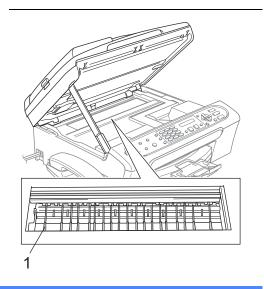
Clean the machine printer platen (1).
