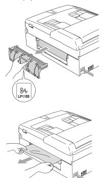
5 Put the Jam Clear Cover back on. Make sure the cover is set properly.
