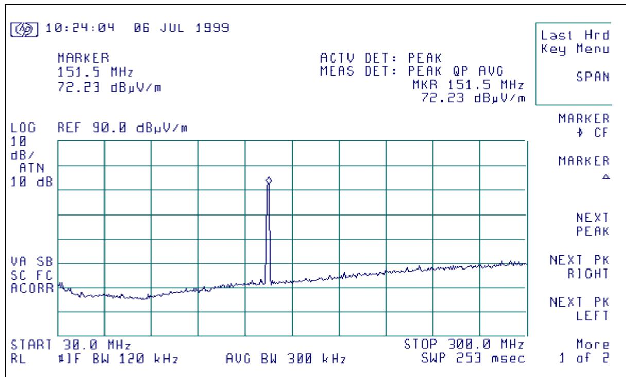
Radiated Emissions signature scan, 162 MHz, vertical polarity, 500 milliwatt level, 30-300 MHz
