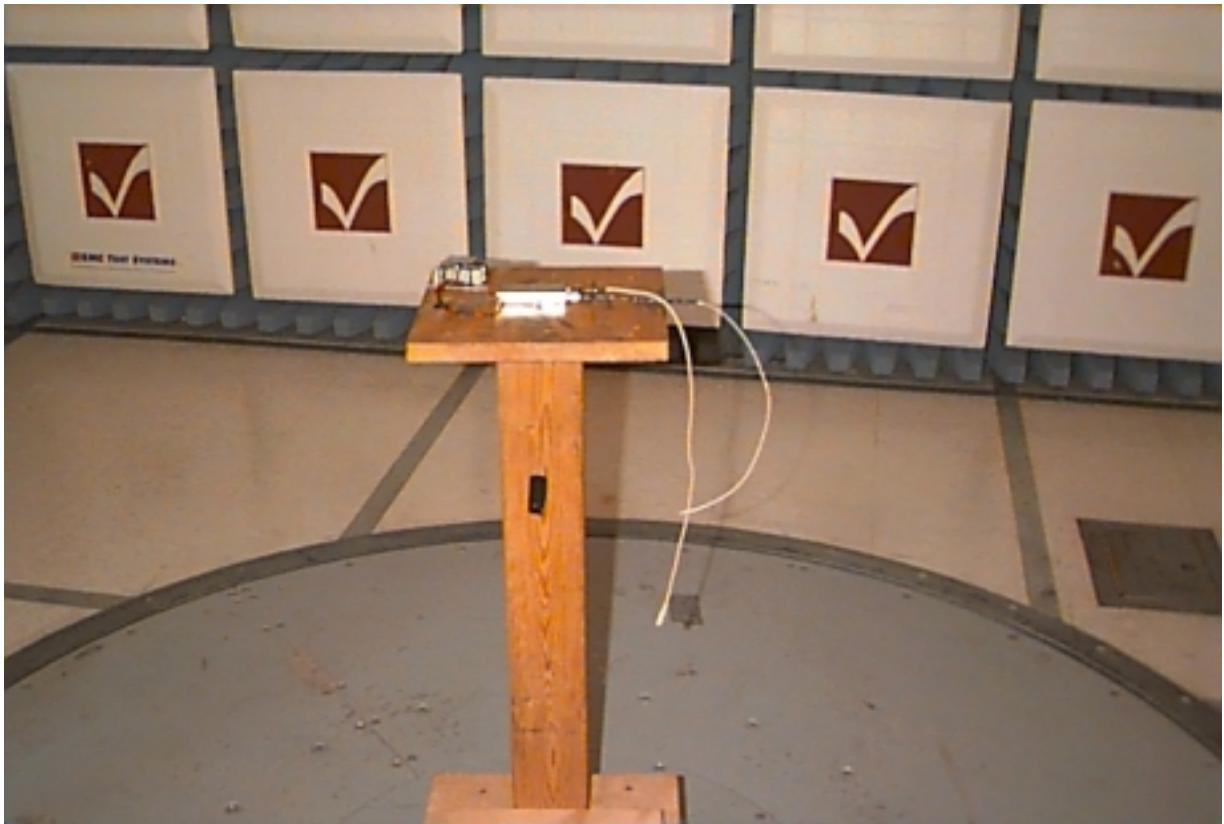
view shows 270 degree position with unit flat, microphone connected, antenna physically attached, but dummy load internally connected to transmitter output
