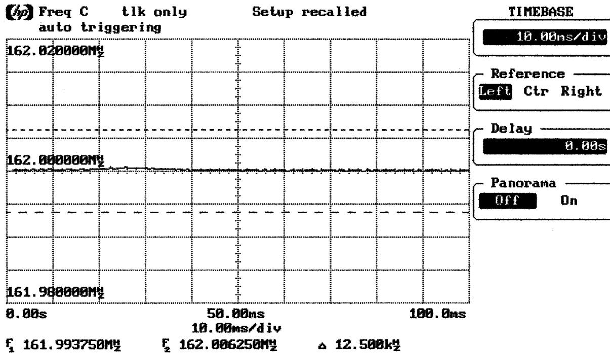
Test Condition: 162 MHz, 250 mW. Frequency Up to 100 ms
