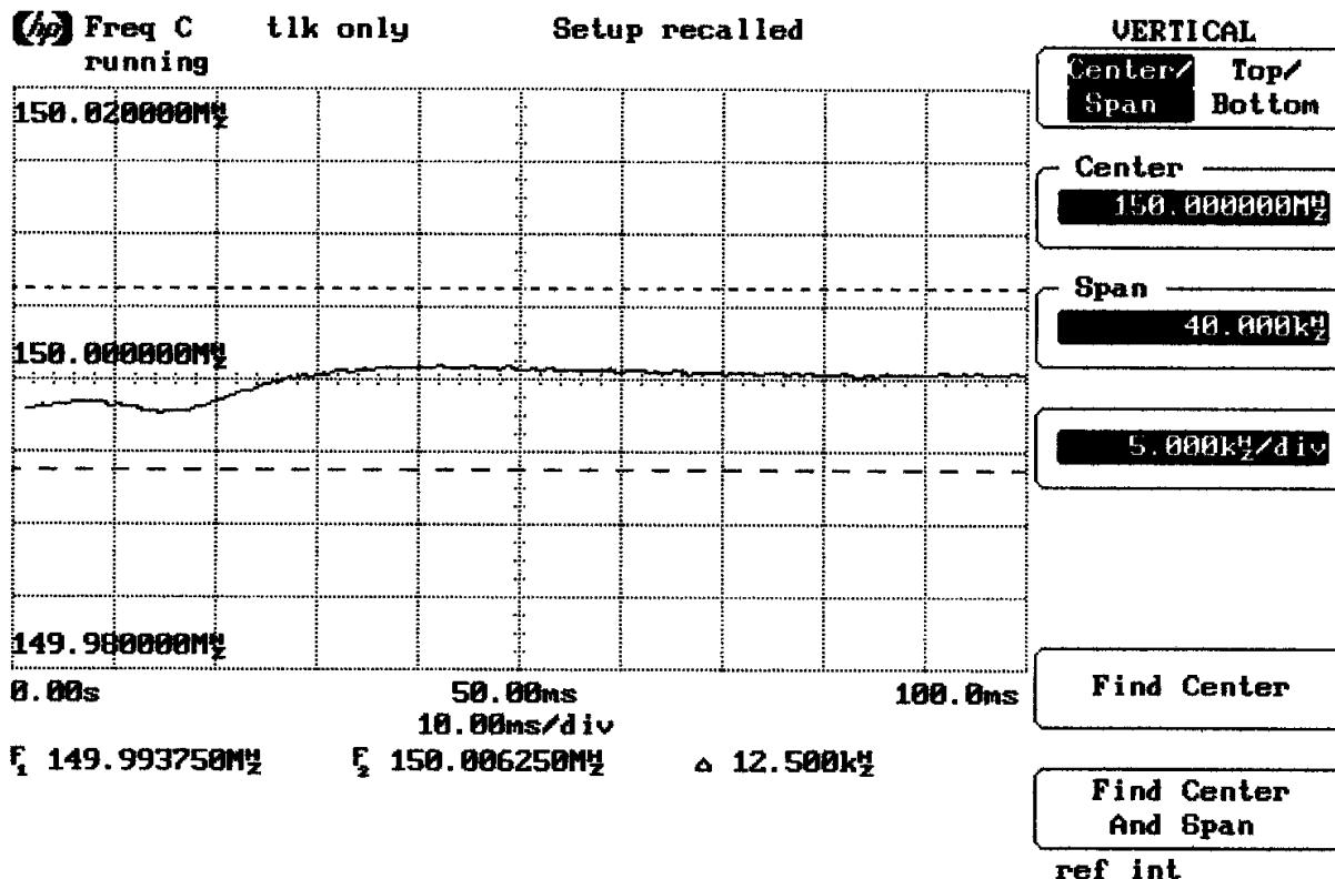
Test Condition: 150 MHz, 250 mW. Frequency Up to 100 ms
