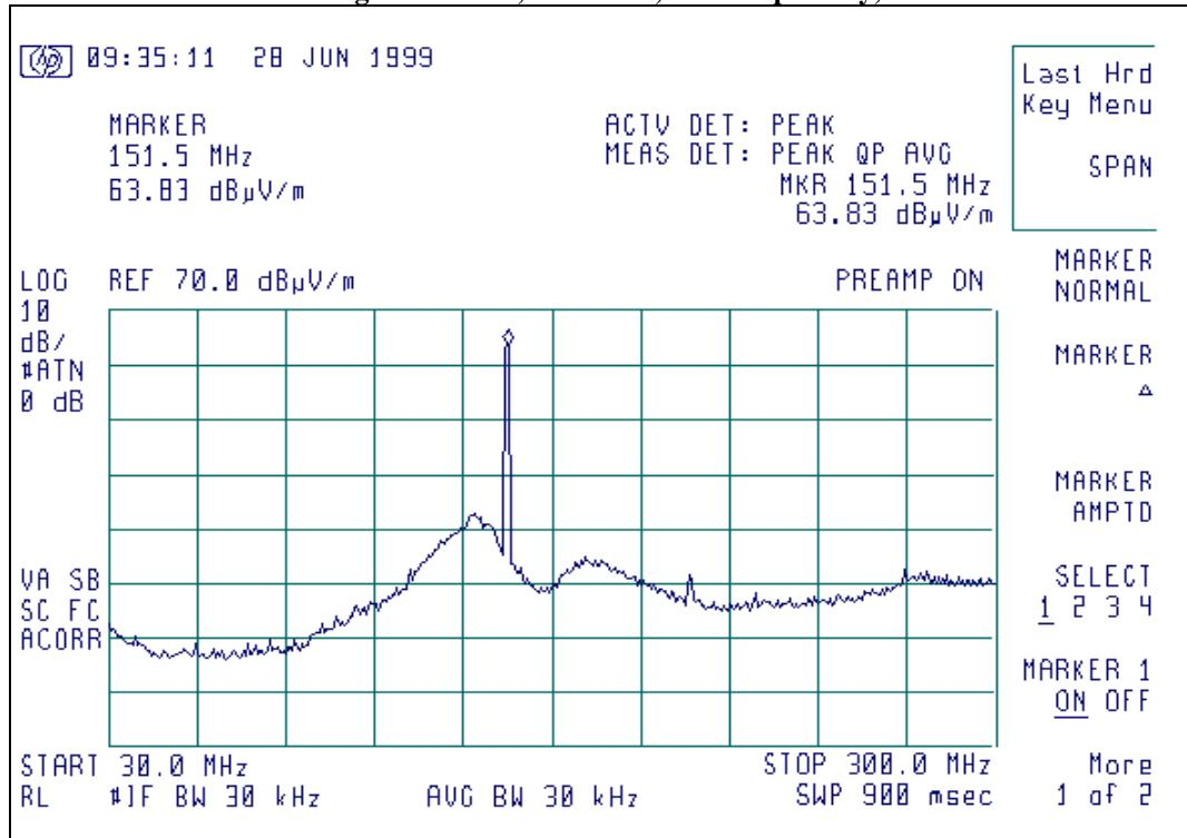
Radiated Emissions signature scan, 162 MHz, vertical polarity, 250 milliwatt level.
