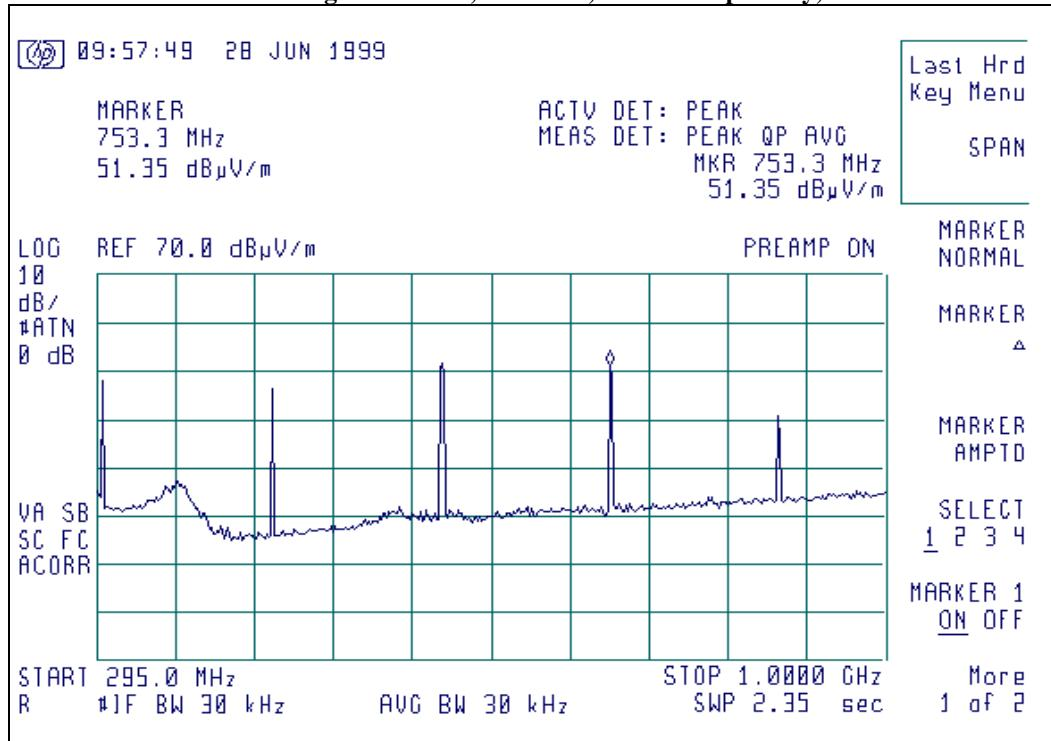
Radiated Emission signature scan, 150 MHz, horizontal polarity, 250 MW level
