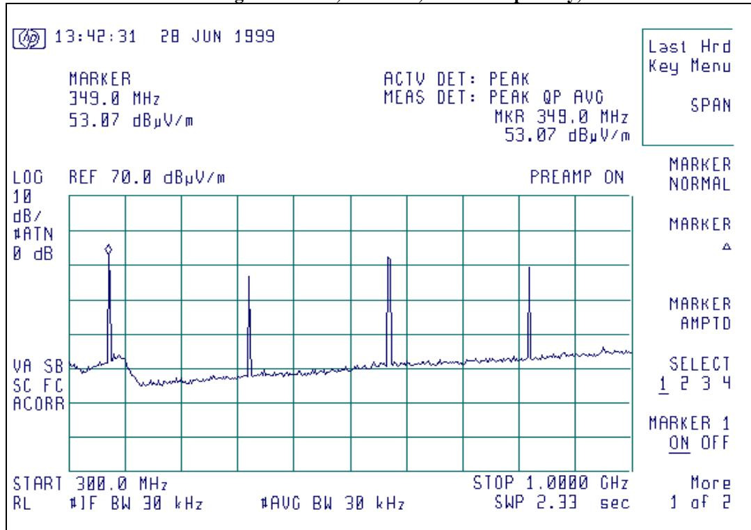
Radiated Emission signature scan, 174 MHz, vertical polarity, 250 MW level
