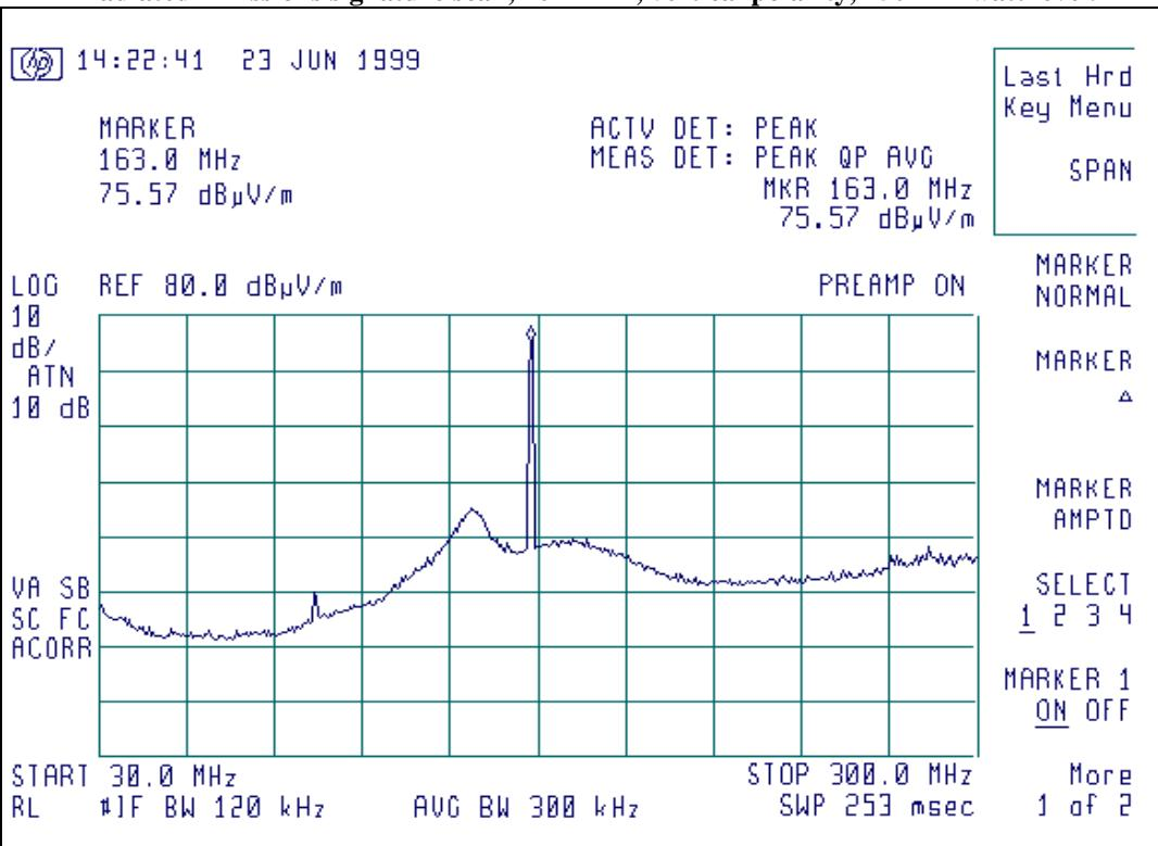
Radiated Emission signature scan, 174 MHz, vertical polarity, 250 MW level
