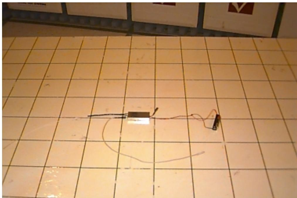
view shows 0 degree position with unit in flat, microphone connected, antenna physically attached, but dummy load internally connected to transmitter output
