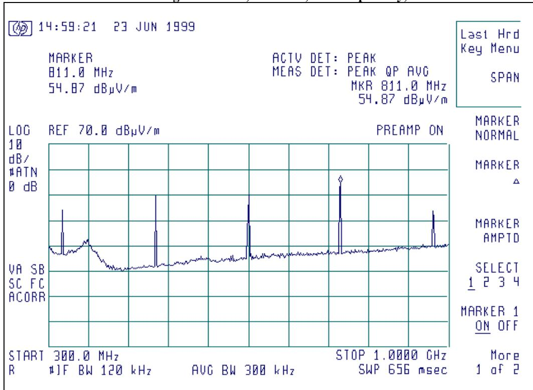
Radiated Emission signature scan, 162 MHz, vertical polarity, 250 MW level
