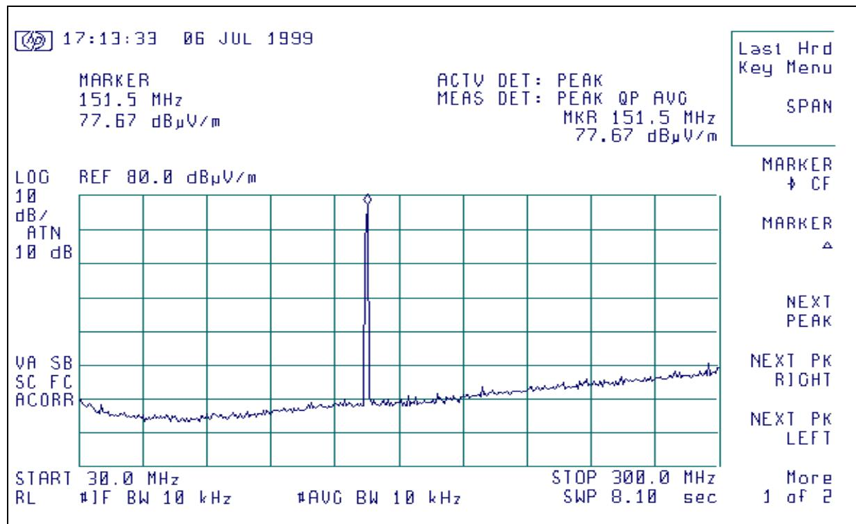
Radiated Emissions signature scan, 162 MHz, horizontal polarity, 1000 milliwatt level, 30-300 MHz
