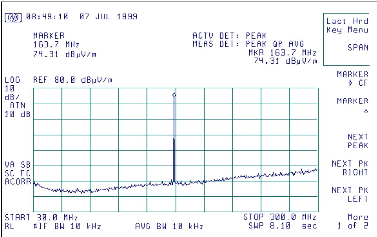
Radiated Emission signature scan, 174 MHz, horizontal polarity, 1000 MW level, 30-300 MHz
