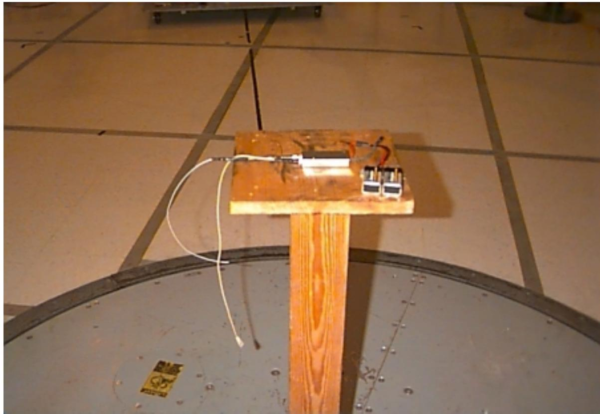
view shows 270 degree position with unit flat, microphone connected, antenna physically attached, but dummy load internally connected to transmitter output.
