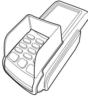
Figure 18 Installed Privacy Shield
