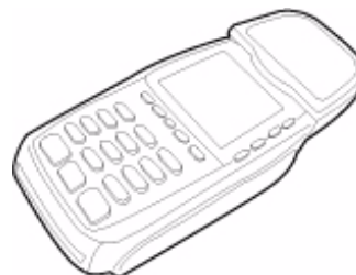
Figure 9 Installed SDIO Contactless Module
