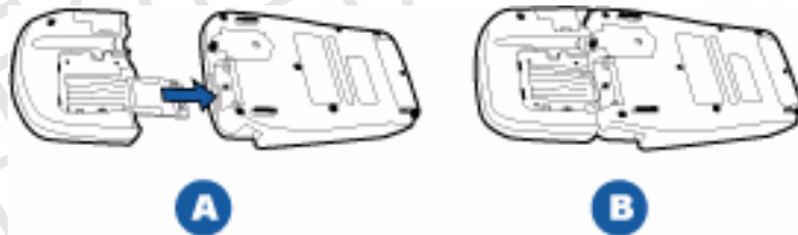
Figure 7 Sliding the RFID Canopy
