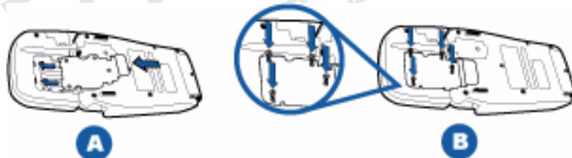
Figure 8 Installing the Metal Plate
