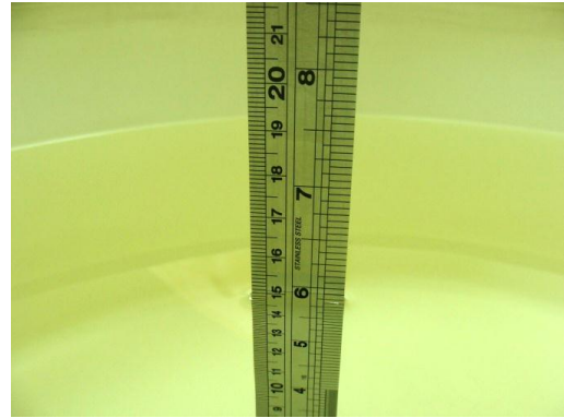
Fig 6.2 Photo of Liquid Height for Body SAR
