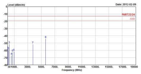
Site : 966 Chamber 5 Condition : PART22/24 3m EIRP\_RSE \_1G~19G HORIZONTAL
