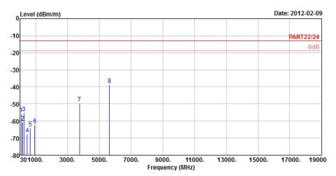
Site : 966 Chamber 5 Condition : PART22/24 3m EIRP\_RSE \_1G~19G VERTICAL
