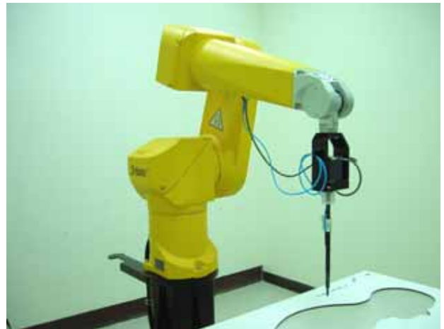
Fig. 5.2 Probe setup on robot
