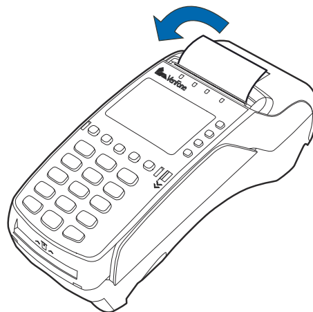
Figure 10 Closing Paper Roll Cover
