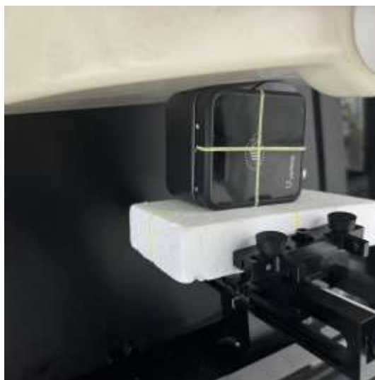
Right Side + Charging Base, Test Separation 0 mm
