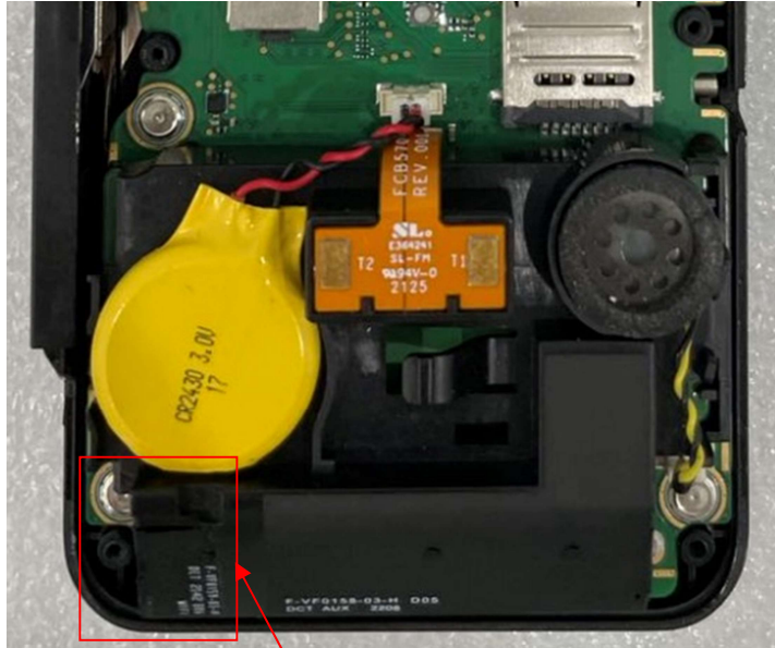
WiFi antenna location
