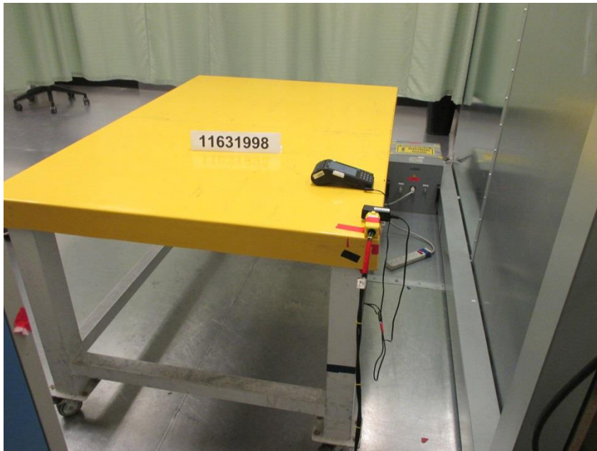
LINE CONDUCTED EMISSION (REAR)
