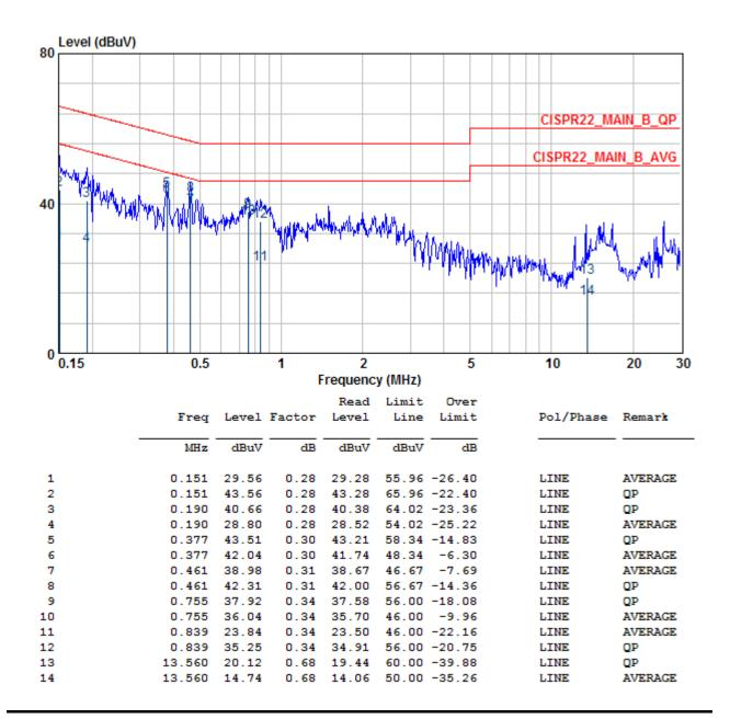
Test Mode : Mode 1, Continuous Transmitting, with antenna
