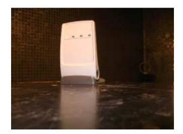
Photograph No.2 Setup for spurious emission field strength measurements in anechoic chamber below 30 MHz
