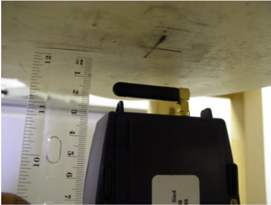
Top Side 1.5cm Separation to Flat Phantom View I
