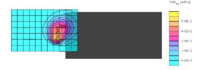
Verifone, Omni5600(CDMA1900, Top Side of the DUT faced toward and 1.5cm separation with flat phantom, Antenna 1, Ambient Temp = 23 Deg C, Liquid Temp = 22 Deg C, 8/4/04)
