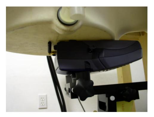
Back Side 1.5cm Separation 1900MHz (Antenna 2)
