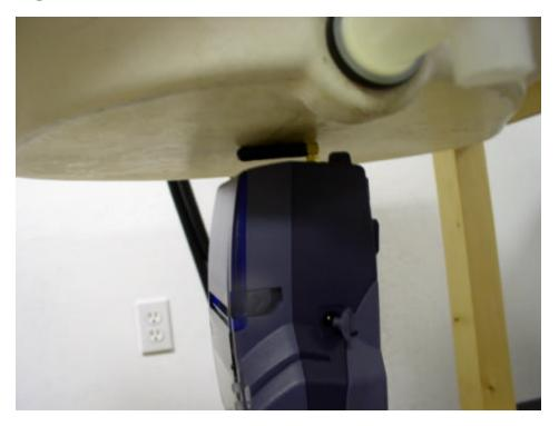
**Top Side 1.5cm Separation 1900MHz (Antenna 2)**
