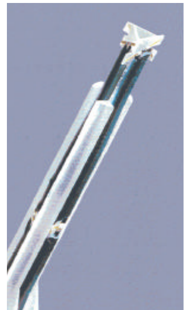
Inside view of ES3DV2 E-field Probe
